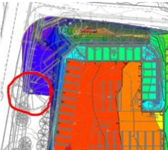
Figure 17 (left)- The large Ash tree highlighted by a red circle would also be subjected to excavations underneath the RPA and trunk of up to -0.75m
